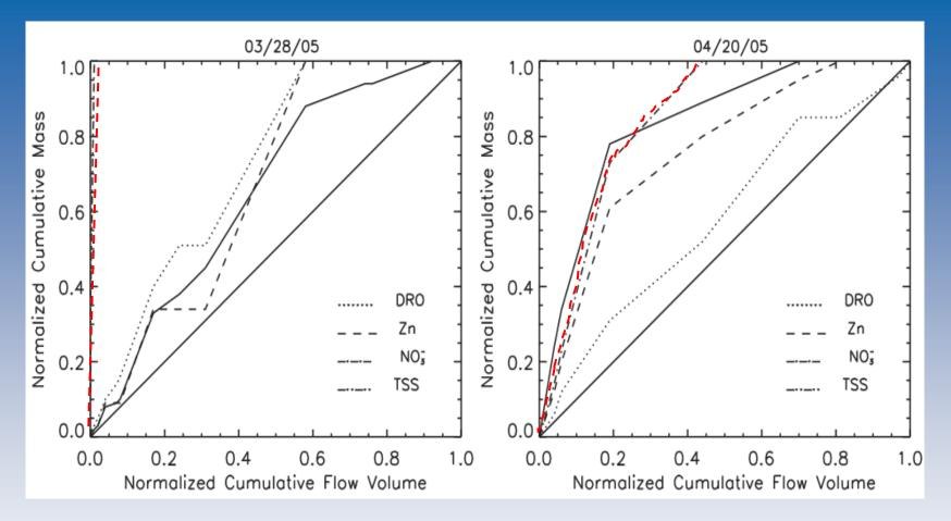
Mass loading for DRO, Zn, NO3, TSS as a function of normalized storm volume for two storms: (a) a large 60 mm rainfall over 1685 minutes; (b) a smaller 15 mm storm depth over 490 minute. DRO=diesel range organics, Zn= zinc, NO3= nitrate, TSS= total suspended solids
