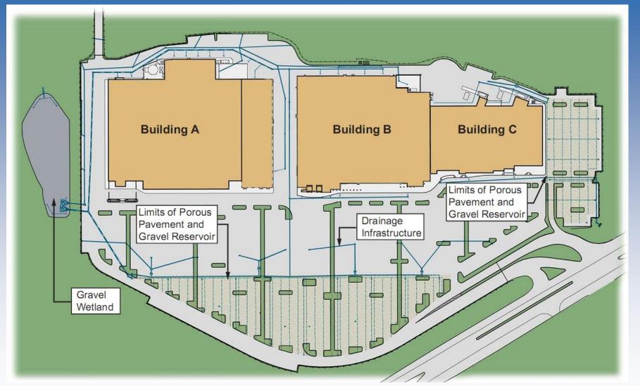
28 ac site, initially >95% impervious, now <10%EIC, with all drainage through filtration, expected to have minimal WQ impact except thermal and chloride
