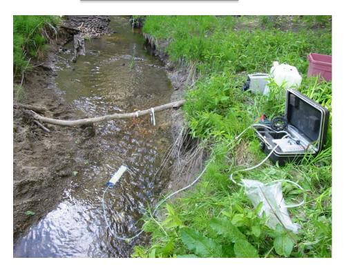
➤ Combined NH<sub>4</sub>+/PO<sub>4</sub><sup>3-</sup> solute addition using Br<sup>-</sup> and Rhodamine as tracers
