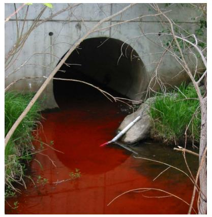
➤Upstream-Downstream O<sub>2</sub> change w/reaeration determined using SF<sub>6</sub>
