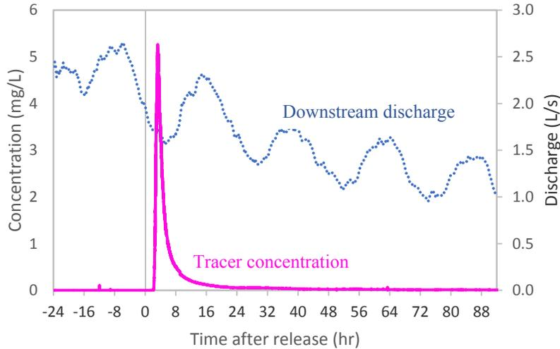
*Figure 3. Continuous breakthrough curve of rhodamine WT (RWT) tracer concentration measured at the outlet of wetland study site BAR from June 18-23, 2014. The peak tracer concentration reached the outlet 3.5 hours after the release. Half of the dye exited by 9.7 hours. Discharge generally declined during the steady period.*
